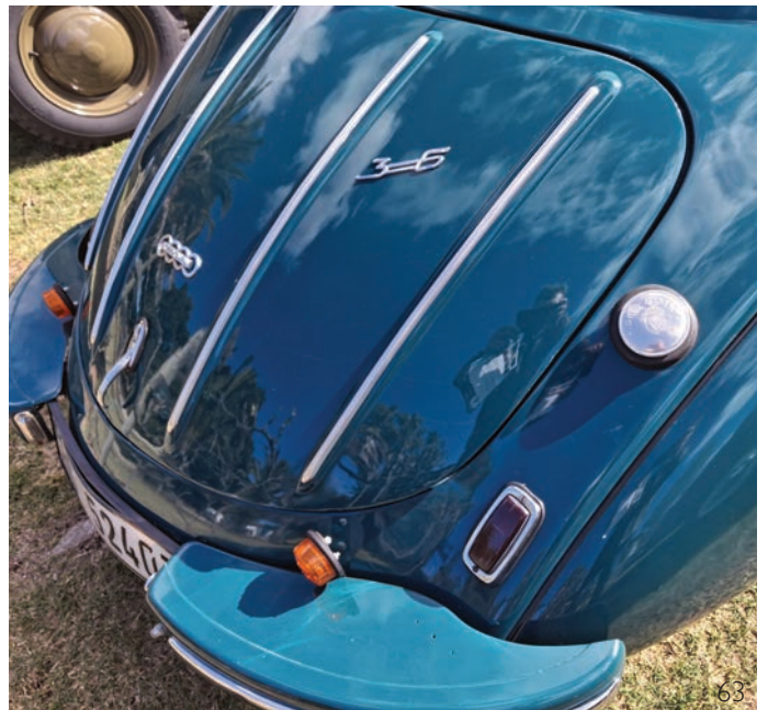
Removing the grille gives access for ignition points adjustment.
