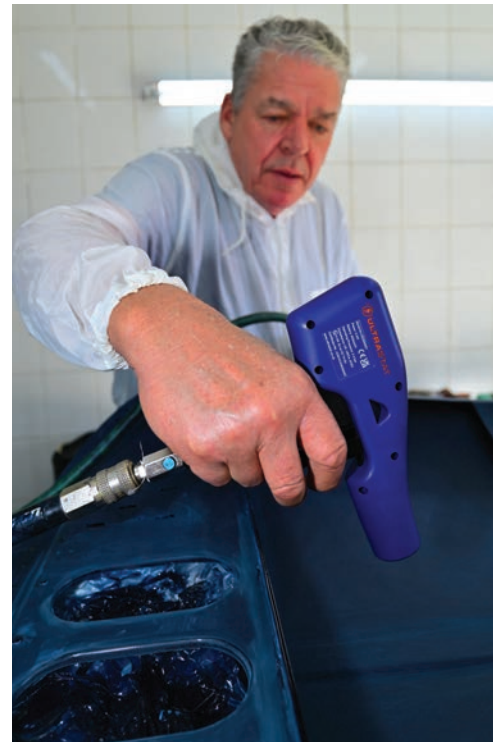
Working like a normal blow gun, the UltraStat creates an ionic air curtain that stops static dust attraction.
